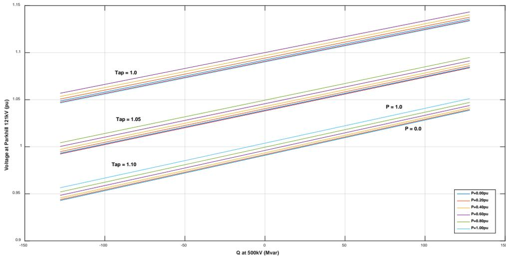
**Figure 6. Variation in Main Substation 121 kV Voltage vs. Reactive Power Supply for a 500 kV Voltage of 1.09 pu**
