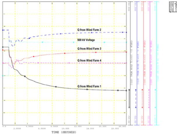
**Figure 12. Reactive Responses of the Four Wind Farms When Controlling Their Local 121 kV Voltages**
