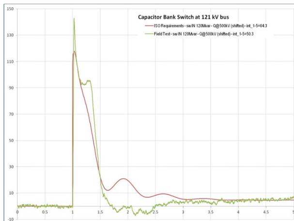
**Figure 9. Comparison of the Wind Farm Response to a Staged Test and the ISO Requirement**
