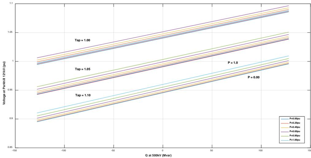
**Figure 8. Variation in Main Substation 121 kV Voltage vs. Reactive Power Supply for a 500 kV Voltage of 1.04 pu**
