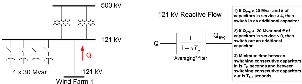
Figure 4. Control Logic for the Four 121 kV 30 Mvar Capacitor Banks
