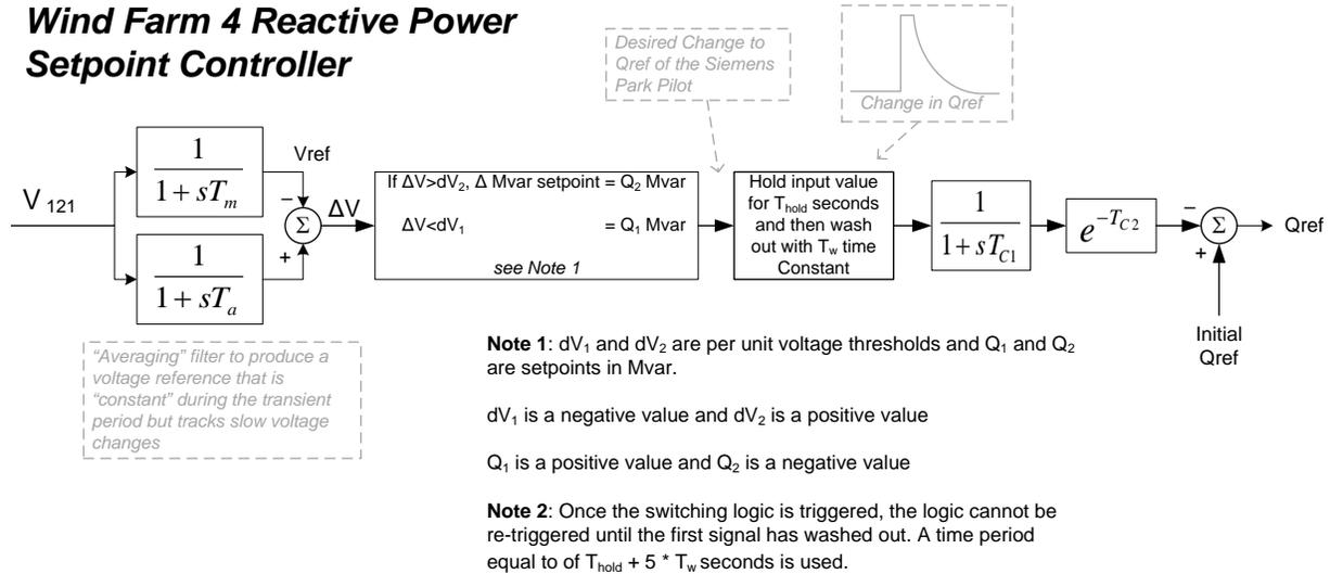
**Figure 2. Block Diagram of Wind Farm 4 Reactive Power Setpoint Controller**
