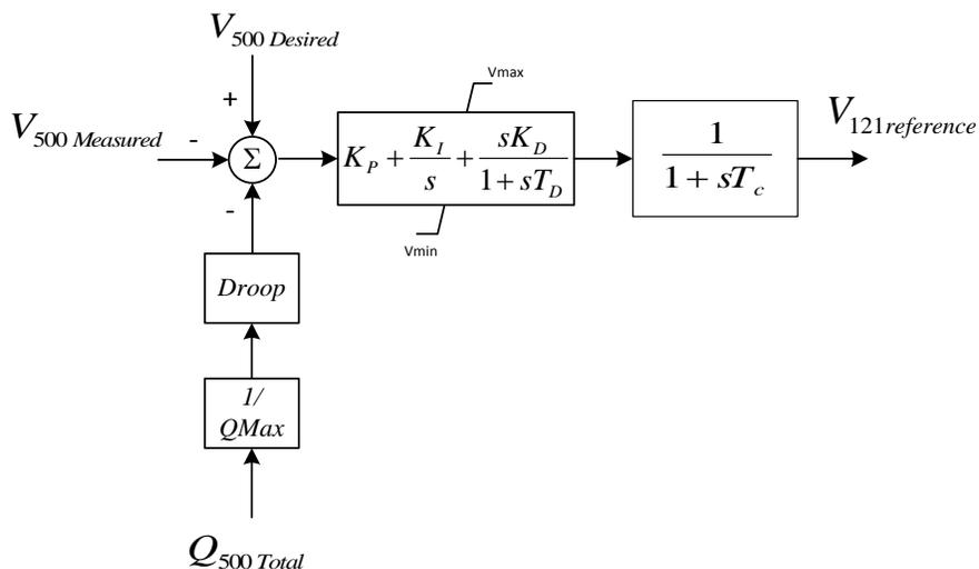
**Figure 3. Outer Loop Controller to Adjust the Reference Voltage of the GE WindCONTROL Controller to Implement the Reactive Power Droop at the 500 kV Bus**
