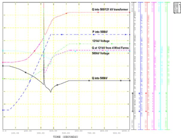
**Figure 11. Control Response Due to a Ramp in Power**
