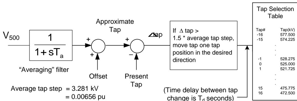
**Figure 5. Control Logic of the Two 525/121 kV Autotransformer’s OLTC’s at the Main Substation**
