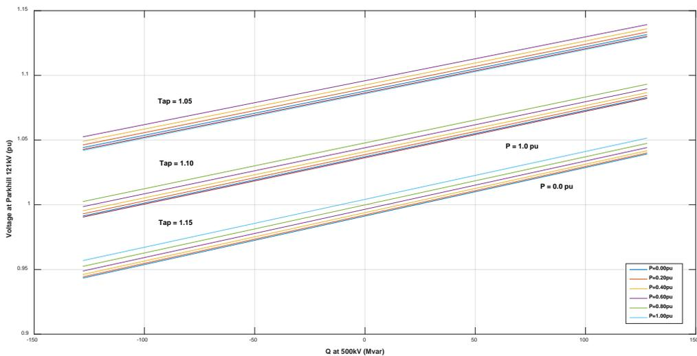
**Figure 7. Variation in Main Substation 121 kV Voltage vs. Reactive Power Supply for a 500 kV Voltage of 1.14 pu**
