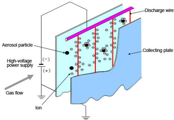
Figure 2: Schematic of electrostatic precipitator
