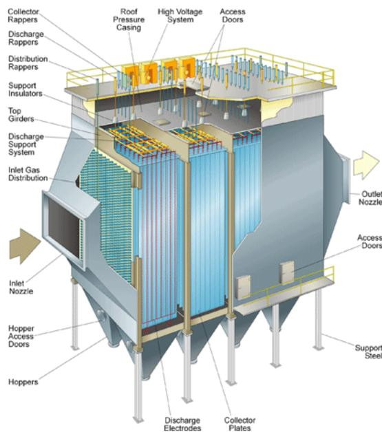
Figure 3: Typical arrangement for Electrostatic Precipitator
