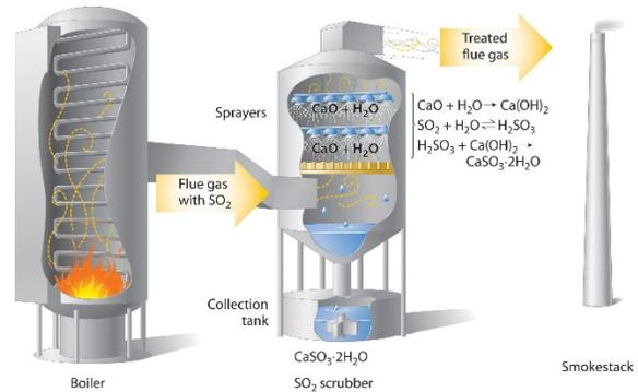
Figure 6: Internal view of generic wet scrubber
