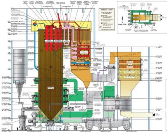
Figure 8: Cross-section view of DFS showing SCR in flue gas path
