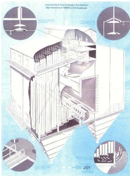
Figure 5: Expanded view of baghouse at AVS
