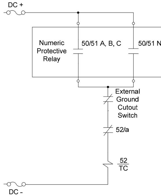
Figure 5. Miswired Simple Overcurrent Scheme
