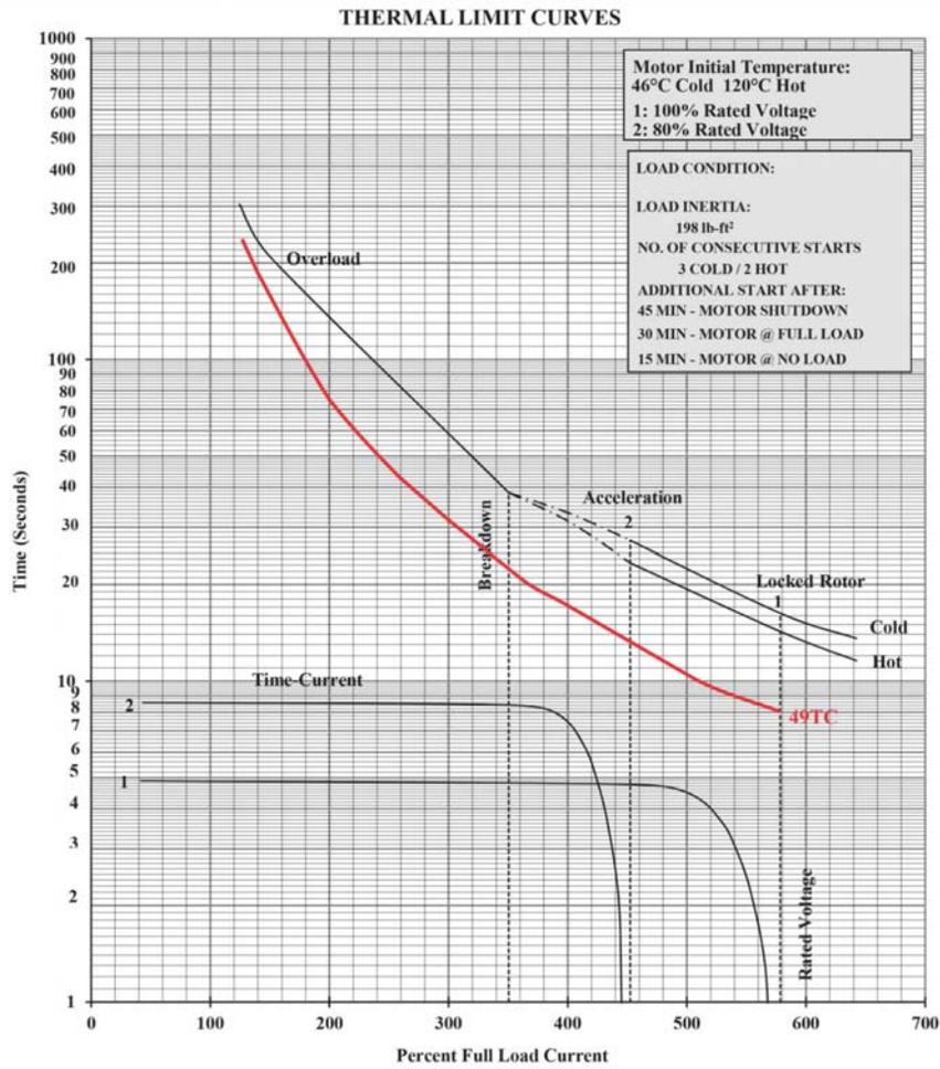
Figure 3. Motor Thermal Limit vs. Programmed 49TC
