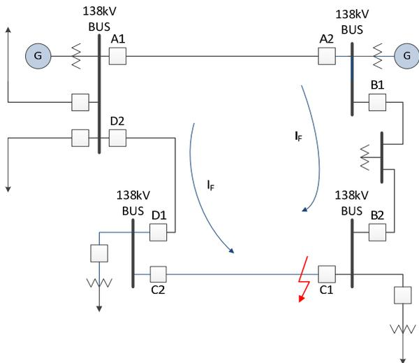
**Figure 8: Single-Line of a Tightly Looped System**
