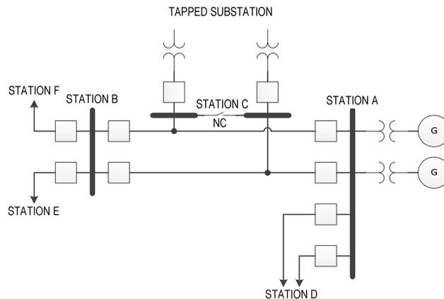
**Figure 9: Single-Line of a Multi-Terminal Line**
