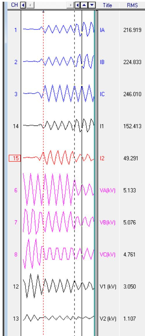
Figure 8 – Evolving Fault, Phase-to-Phase to Three Phase
