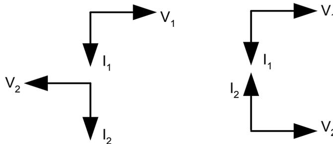
Figure 5B – Symmetrical Component Voltage and Current Phase Relationships
