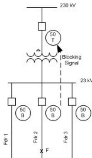
Figure 6 – Distribution Bus Bar Blocking Scheme – Fast Bus Trip
