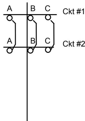
Figure 1 – Three Phase Fault on Double Circuit Distribution Line
