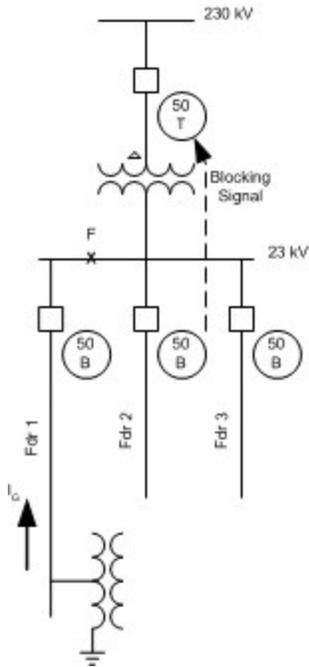
**Figure 7 – Ground Source Connected to Distribution Feeder**
