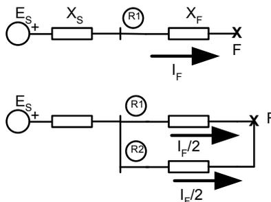
Figure 2 – Double Circuit Distribution Fault Analysis
