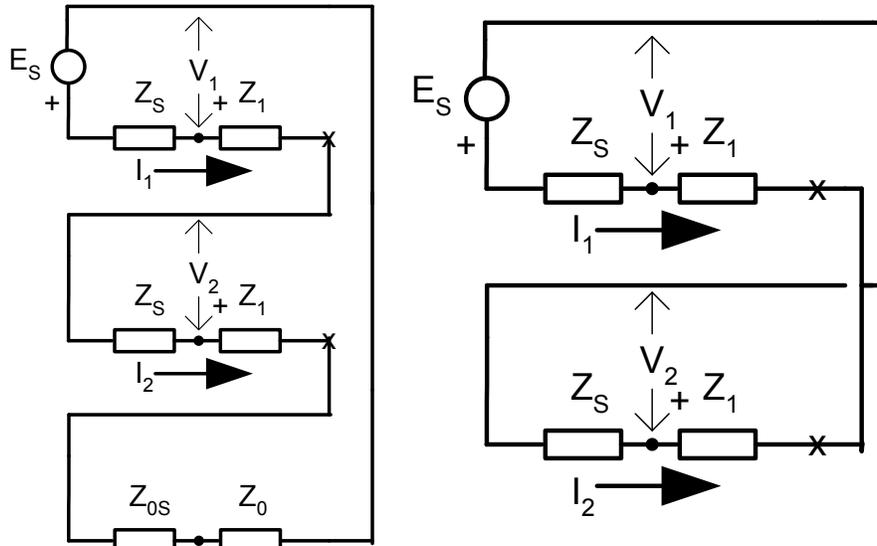
Figure 5A – Symmetrical Component Diagrams for Single Phase-to-Ground and Phase-to-Phase Feeder Faults
