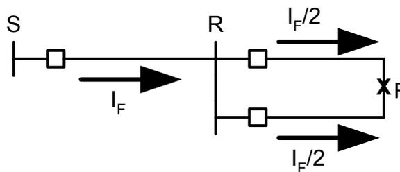
**Figure 3 – Double Circuit Distribution Fault Analysis**
