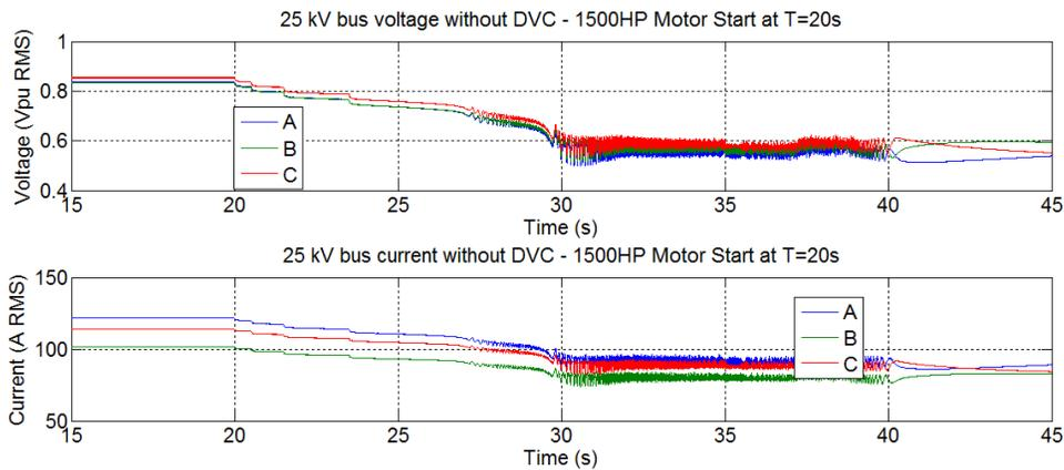
**Figure 5. Motor bus voltage (top) and current (bottom) for the 1500 hp motor start, last to start, without the DVC.**
