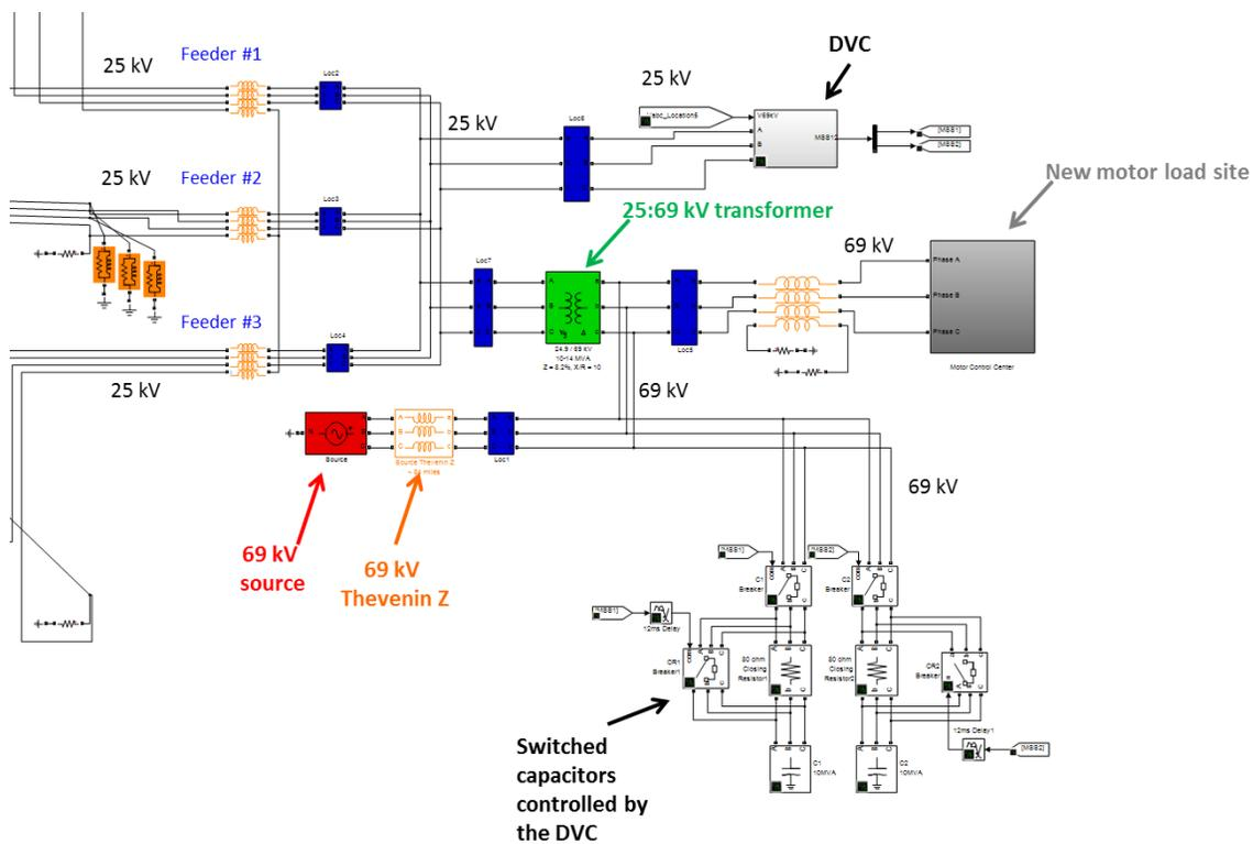
Figure 3. Zoomed version of Figure 2, showing the local substation, DVC, and the new customer site.
