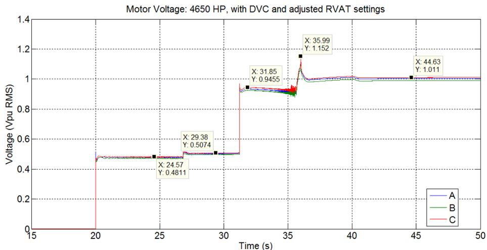
Figure 12. Voltage applied to the terminals of the 4650 hp motor (output voltage of the RVAT).
