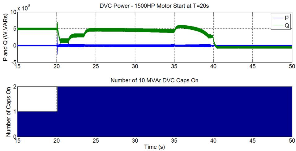
Figure 7. Real and reactive power from the DVC during the 1500 hp motor start, last to start.
