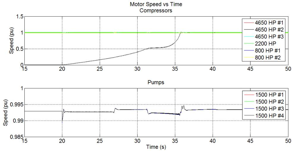
Figure 10. Customer motor speeds in the last-to-start case of the 4650 hp motor, with the DVC and the aggressive RVAT settings.
