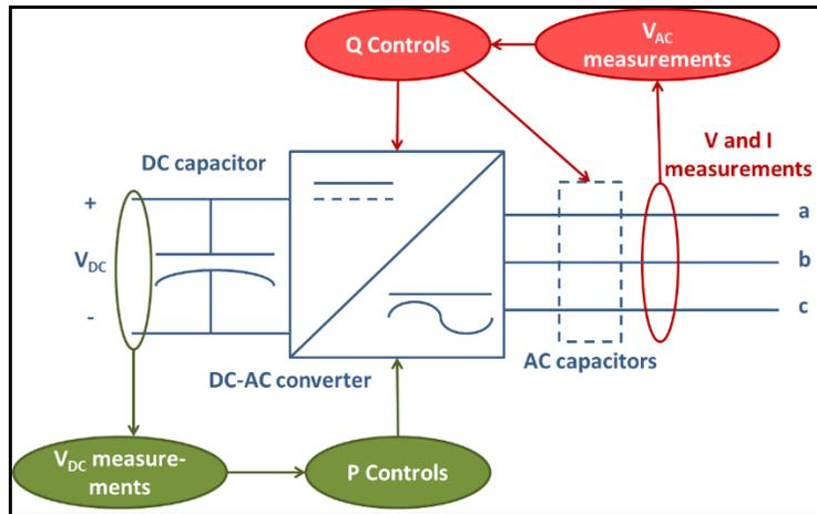
**Figure 1. Simplified block diagram of the DVC.**
