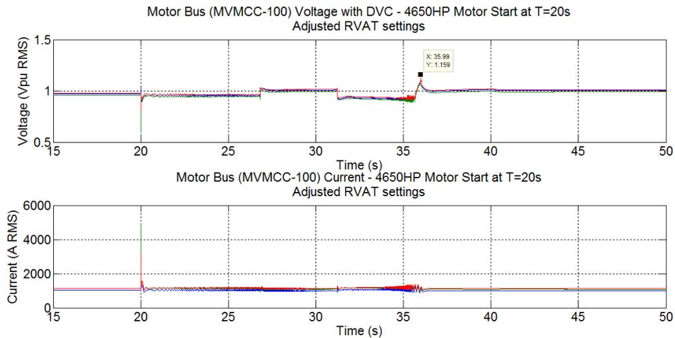
Figure 11. Motor bus voltage (top) and current (bottom) during the 4650 hp last-to-start event, with the DVC and the more aggressive RVAT settings.
