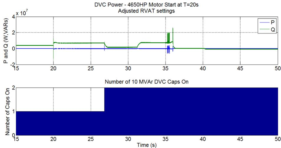
**Figure 13. DVC output power (top) and capacitor status (bottom) during the 4650 hp last-to-start event, with the more aggressive RVAT settings.**
