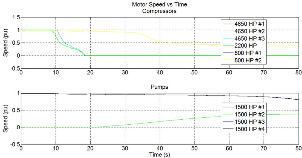
**Figure 4. Speeds of customer motors vs. time for the 1500 hp motor start, last to start, without the DVC.**
