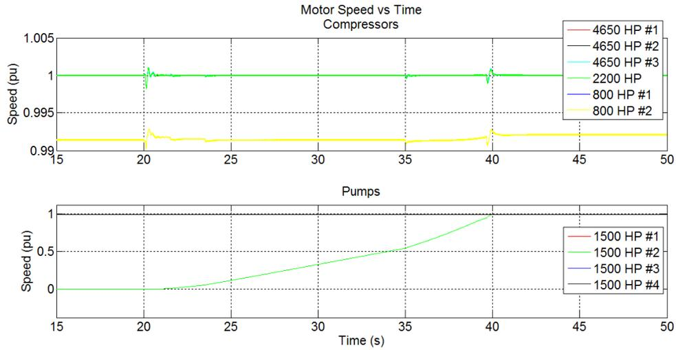
Figure 6. Customer motor speed vs. time for the 1500 hp motor start, last to start, with the DVC.
