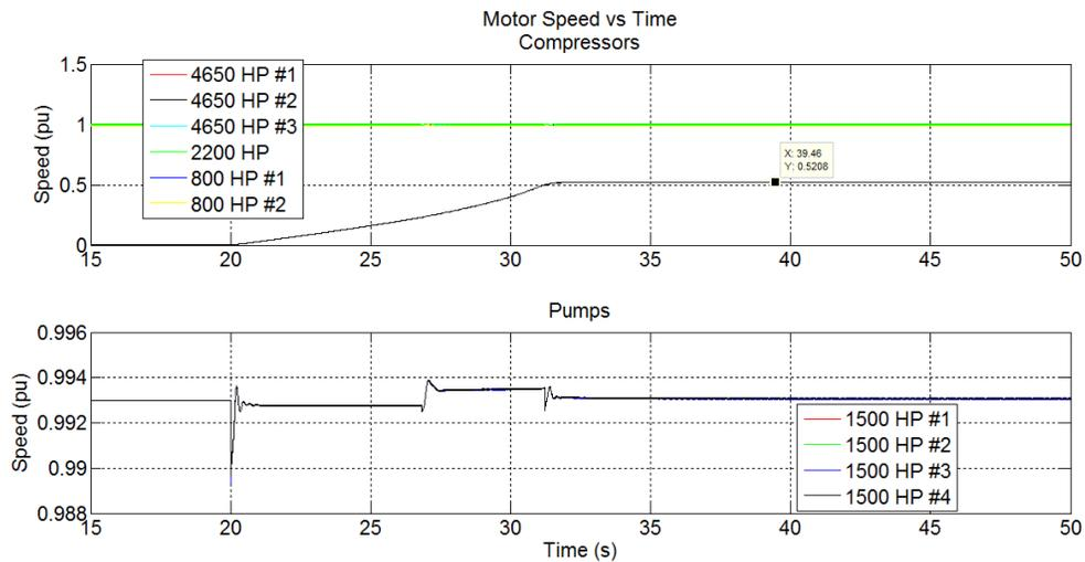
Figure 8. Motor speeds vs. time during the 4650 hp last-to-start event, with the DVC.
