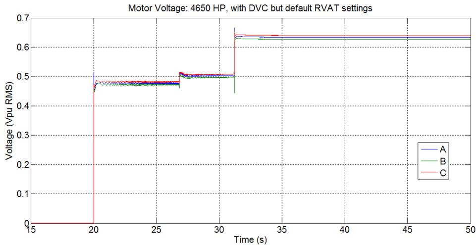
**Figure 9. Voltage at the terminals of the 4650 hp motor (output voltage of the RVAT).**
