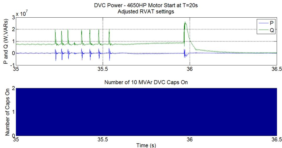
**Figure 14. Zoomed in view of Figure 13, emphasizing the time period between 35 and 36.5 sec when the 4650 hp motor approaches and then reaches synchronous speed.**
