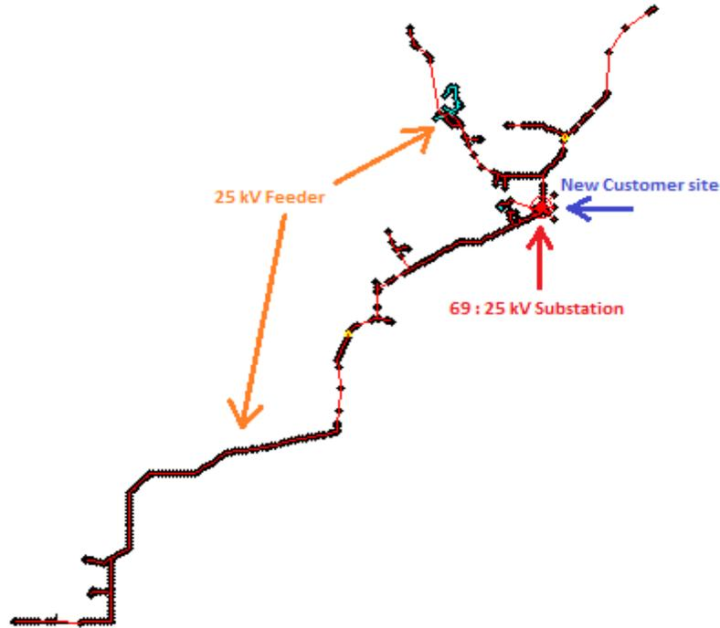
Figure 2. Schematic of the entire model of the local substation, its 25 kV feeders, and the new customer site.
