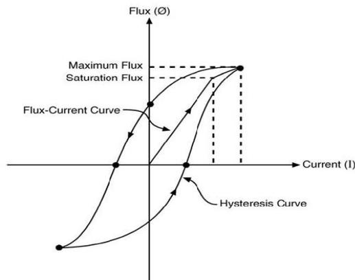
Figure 6: Typical magnetization curve of a power transformer
