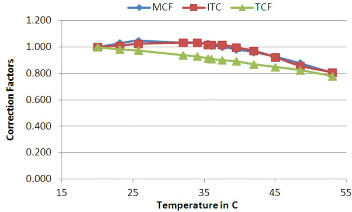
Figure 12: Comparison of ITC and TCF with respect to Measured Correction Factors (MCF) for  $C_{HL}$  insulation
