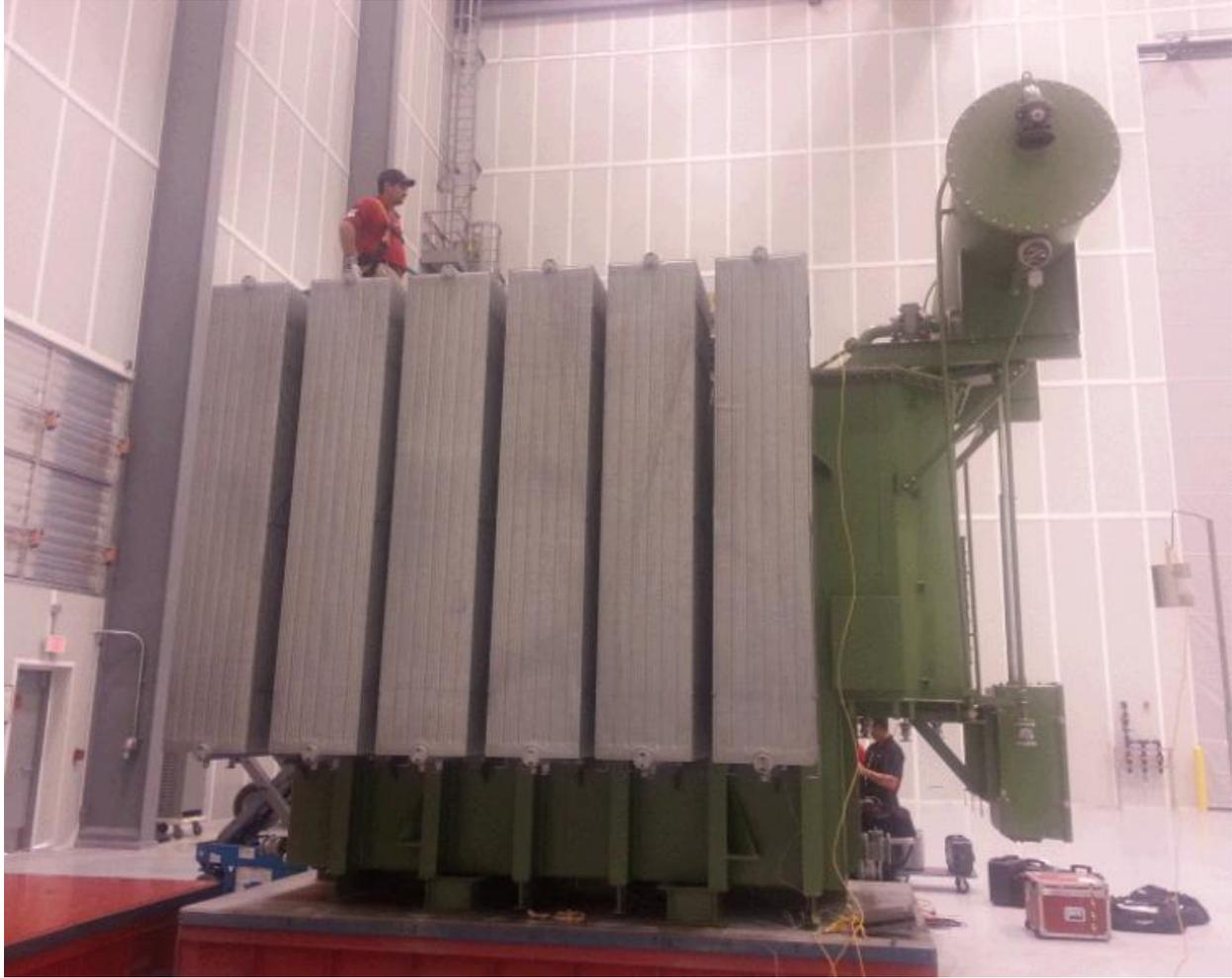
*Figure 9: 40 MVA Delta Wye transformer used as a test object for ITC case study*
