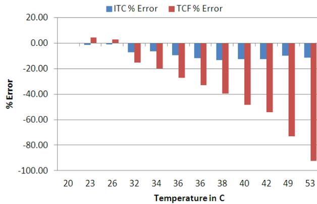
Figure 15: ITC and TCF percent error with respect to Measured Correction Factors (MCF) for  $C_{HG}$  insulation
