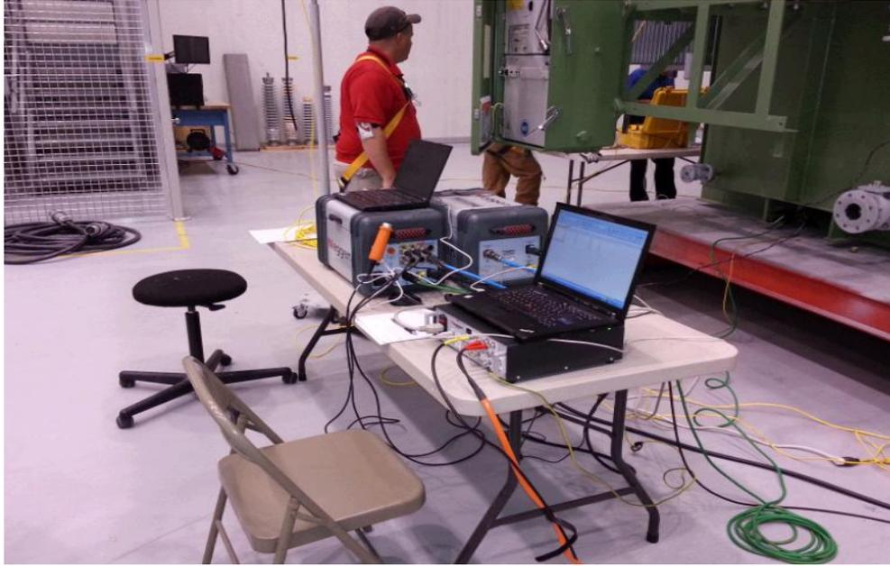
*Figure 11: Test setup to perform Power Factor and DFR tests as transformer cools down*
