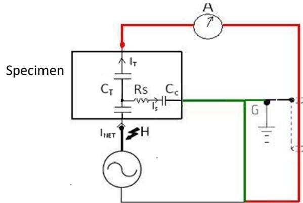
Figure 3: Specimen in UST mode with surface loss components
