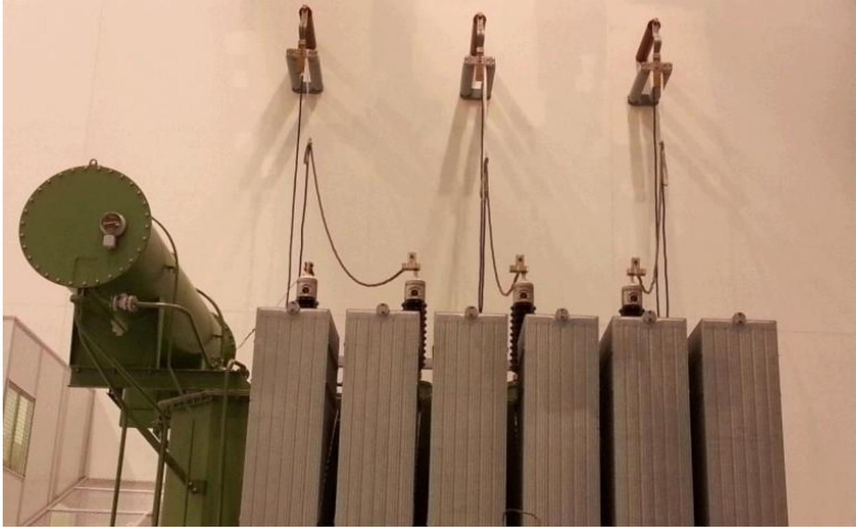
*Figure 10: Windings heated to 75 °C using short circuit method prior to performing the tests*
