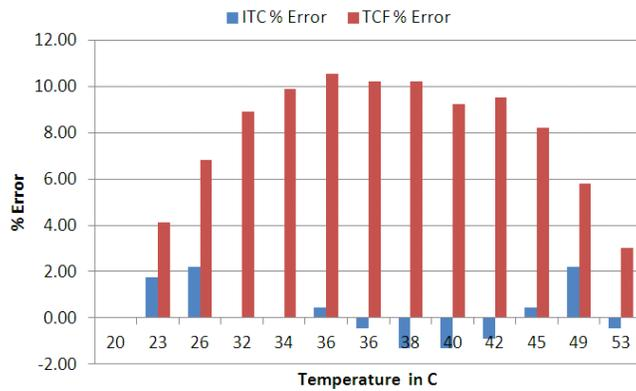
Figure 13: ITC and TCF percent error with respect to Measured Correction Factors (MCF) for  $C_{HL}$  insulation
