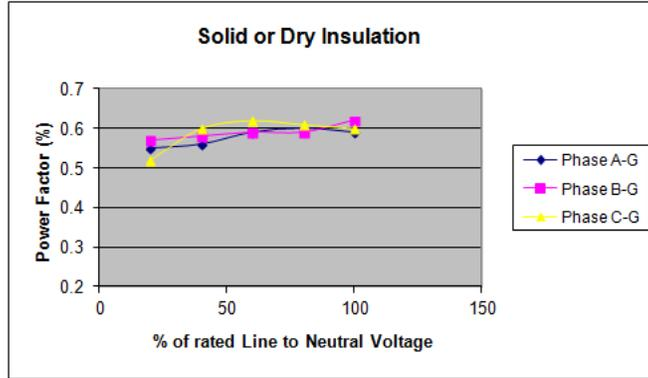
Figure 2: PF measurements as a function of voltage for 2000 HP, 4000V 3- $\Phi$  induction motor
