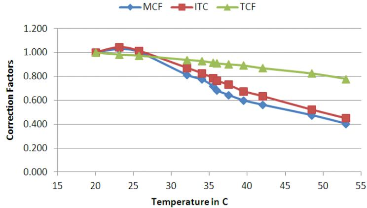
Figure 14: Comparison of ITC and TCF with respect to Measured Correction Factors (MCF) for  $C_{HG}$  insulation
