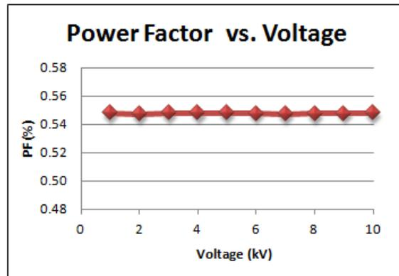
Figure 1:  $C_{HL}+C_{HG}$  PF measurements as a function of voltage for three phase delta delta transformer
