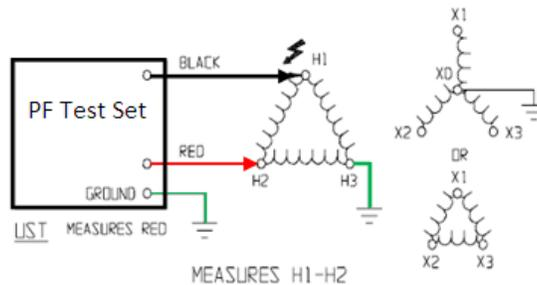
Figure 7: Excitation current measurement on a Delta winding with third leg grounded
