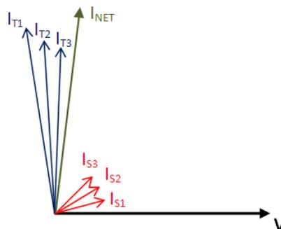
Figure 4: Vector diagram with different  $I_s$  phase angles
