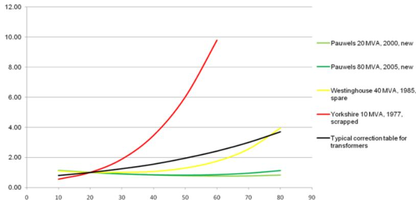
Figure 8: Temperature dependence of different transformers with different levels of ageing
