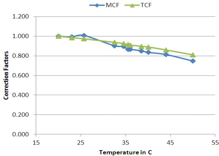
Figure 16: Comparison of MCF and TCF for C<sub>LG</sub> insulation
