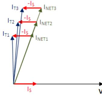
Figure 5: Vector diagram with different magnitude of current  $I_{NET}$  and purely resistive loss current  $I_s$
