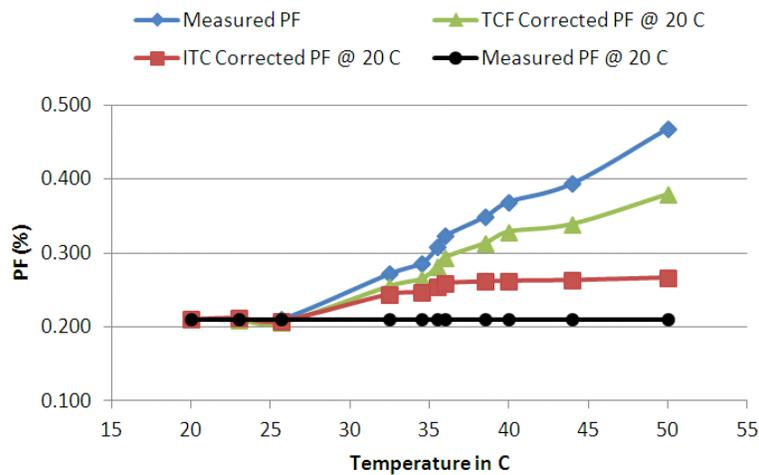
Figure 17: Comparison of ITC and TCF corrected 20 °C values with respect to measured PF readings at different temperatures and 20 °C for C<sub>HL</sub> insulation
