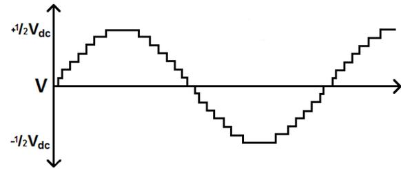
**Fig. 3.** Cascaded Two Level (CTL) Converter Voltage Waveform
