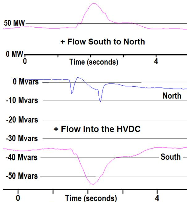
**Fig. 10.** August 27<sup>th</sup> HVDC MW and Mvar Flows Following Loss of a 345 kV Source to the UP.
