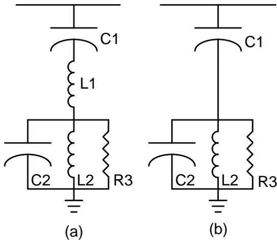
**Fig. 6.** Mackinac HVDC Filters (a) Original 5<sup>th</sup> and 30<sup>th</sup> Harmonic and (b) Modified 5<sup>th</sup> and High Pass
