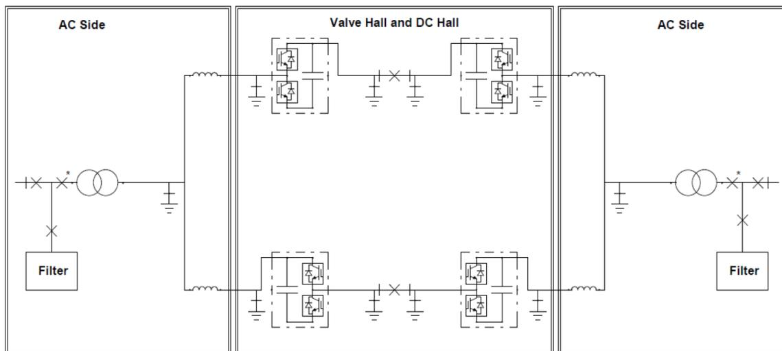
**Fig. 2.** Simplified One-Line Diagram of Mackinac HVDC Converter Station [3]
