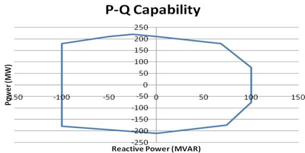
**Fig. 5.** VSC Converters' Capability Curve
