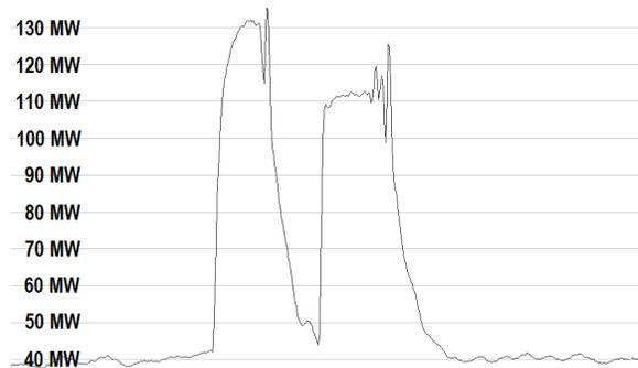
**Fig. 9.** July 16<sup>th</sup> HVDC Power Transfer with Two ~2 Second Deviations from 40 to 130 and 110 MW.
