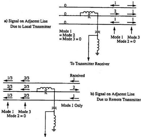
Figure 8: Carrier signal is not confined to coupled phase
