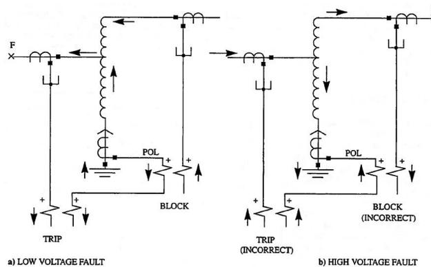
Figure 13: Neutral of autotransformer for polarizing
