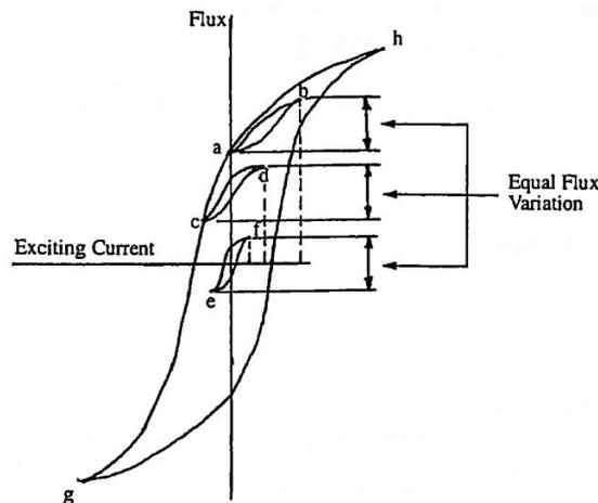
Figure 3: Effect of residual flux on ct exciting current
