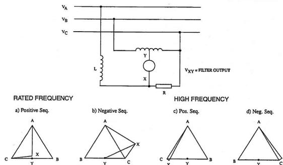
Figure 6: Typical negative sequence filter
