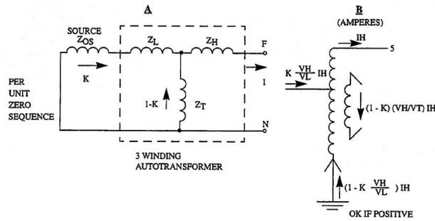
Figure 14: Neutral of autotransformer with delta tertiary for polarizing
