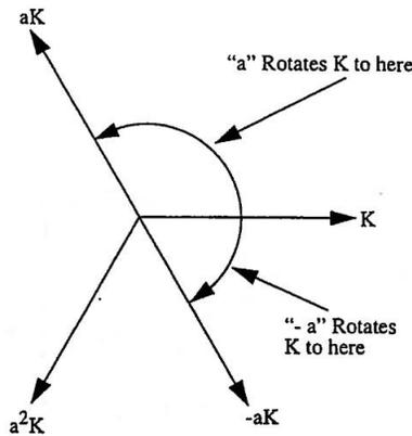
Figure 5: Showing "a" does not rotate a phasor 120° in the clockwise direction.
