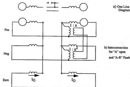
Figure 7: Simultaneous open and  $\phi\phi$  fault
