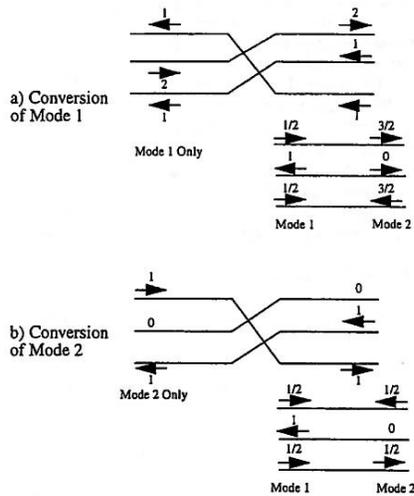
Figure 9: Mode conversion caused by transmission line transposition
