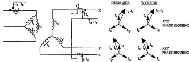
Figure 10: Partial circuit for transformer differential relay showing phase sequence does not matter
