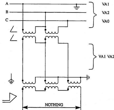
Figure 15: Incorrect use of wye-ground-broken-delta transformer connection
