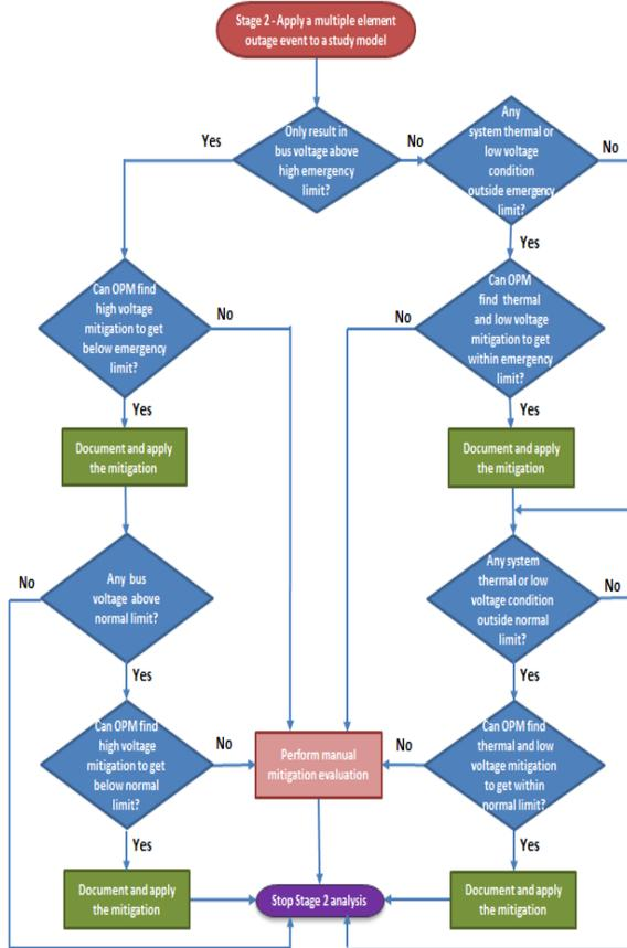
Fig. 2. Stage 2 Flow Chart - Steady State Screening Mitigation Analysis
