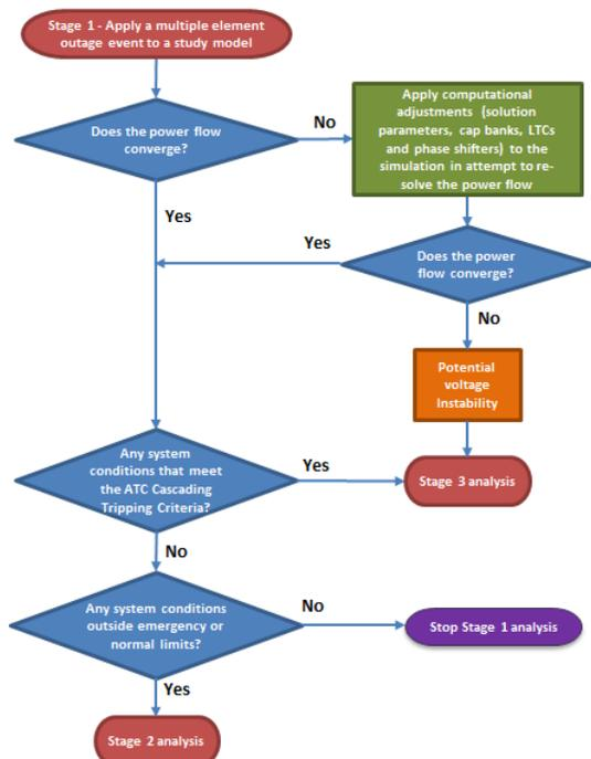
Fig. 1. Stage 1 Flow Chart - Steady State Screening without Mitigation
