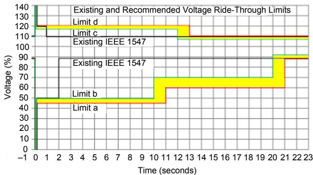
Fig. 2. Existing and proposed voltage ride-through limits.
