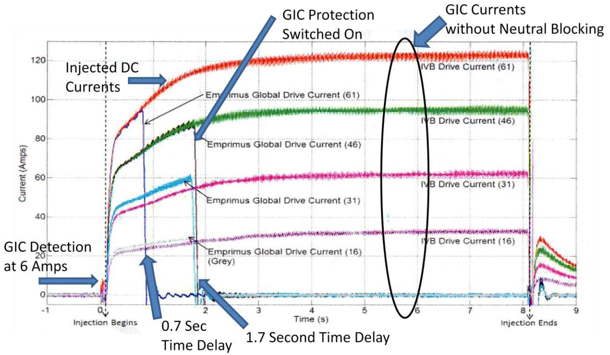
Figure 4 - SolidGround™ Neutral Blocking Live Grid Test Results
