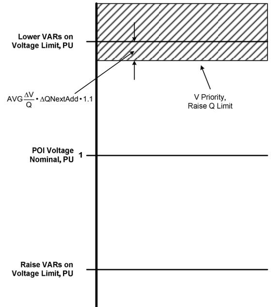
Fig. 3. V priority, raise VARs on Q blocking characteristic
