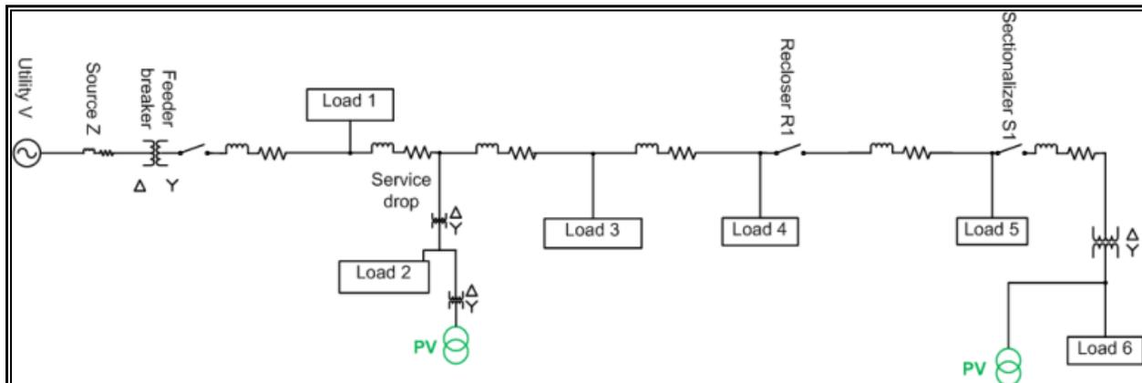
Figure 2. Generalized model of a distribution feeder.
