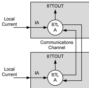
Fig. 2. Multiterminal test concept (Phase A shown)
