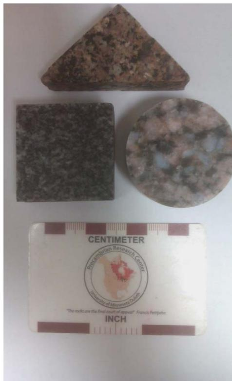
**Figure 5.** Various sample shapes used to measure thermal conductivity in this study.
