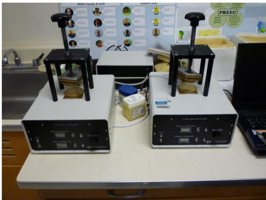
**Figure 6.** PEDB used for measuring thermal conductivity in the UNDGL.
