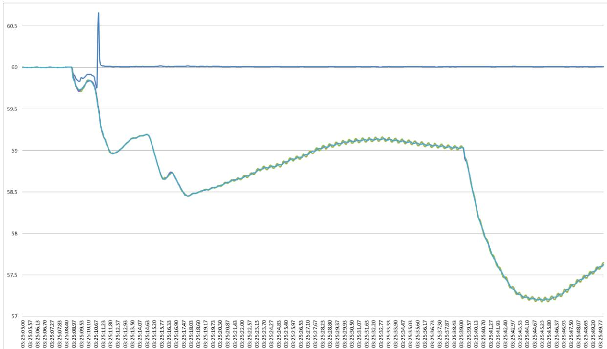
**Figure 3: PMU-recorded frequency data during initial 40 seconds following lightning strike**
