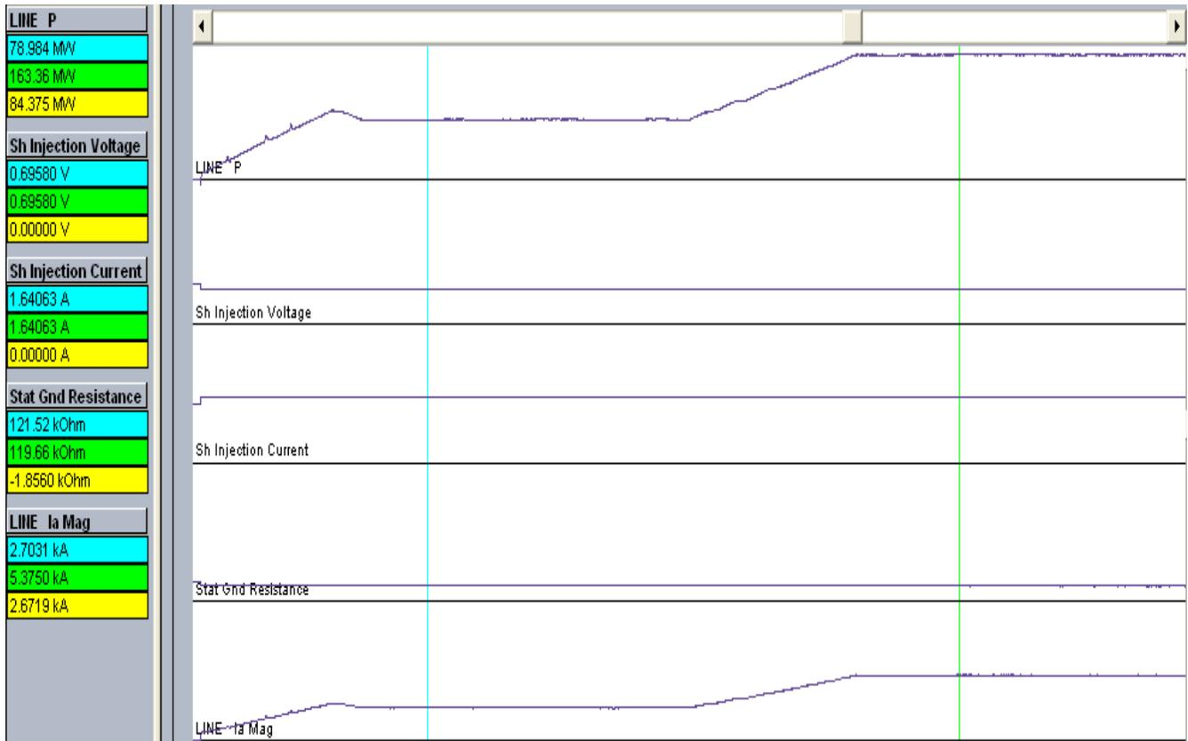
Fig. 10 Data captured for injection module based 100% stator ground protection module at JEA site
