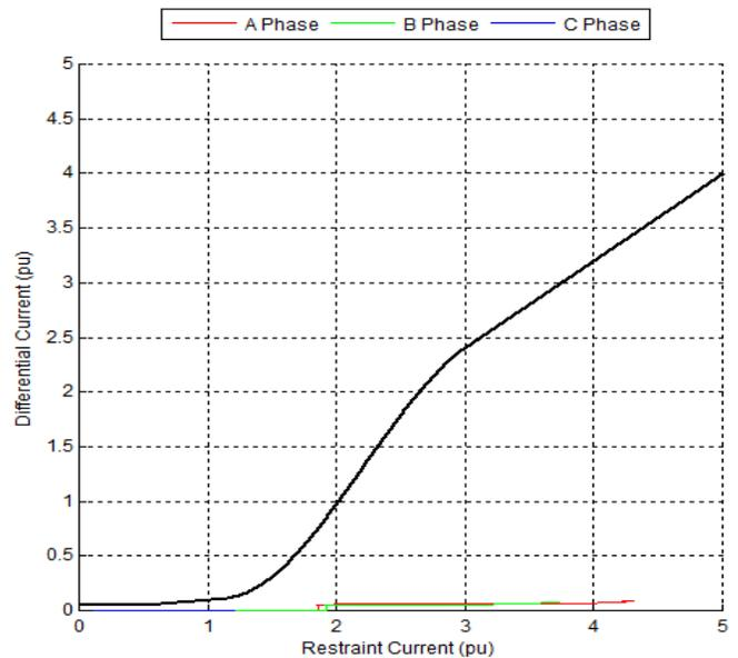
Fig. 3 Three-phase differential protection elements for inter-turn fault in A-phase winding.
