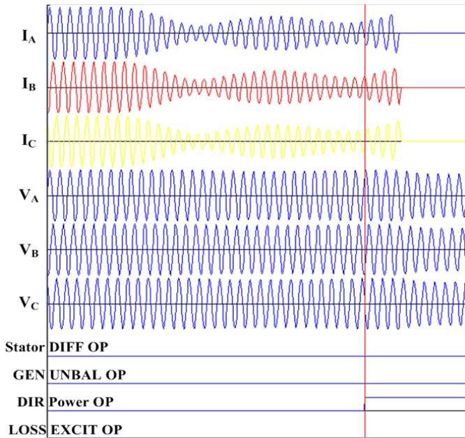
Fig. 6 Captured oscillography from an IED for loss of prime-mover fault
