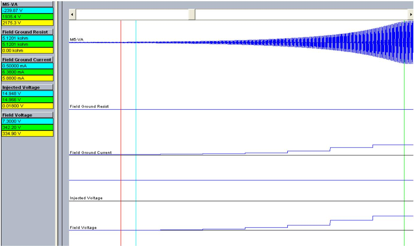
Fig. 9 Data captured for injection module based 100% stator ground protection module.
