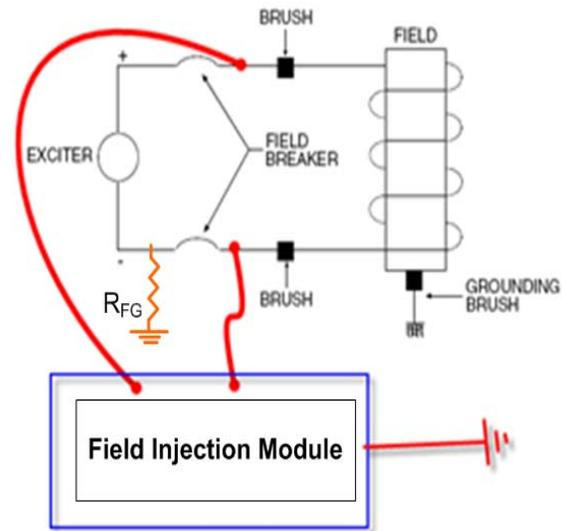
Fig. 8 Field testing setup at site.
