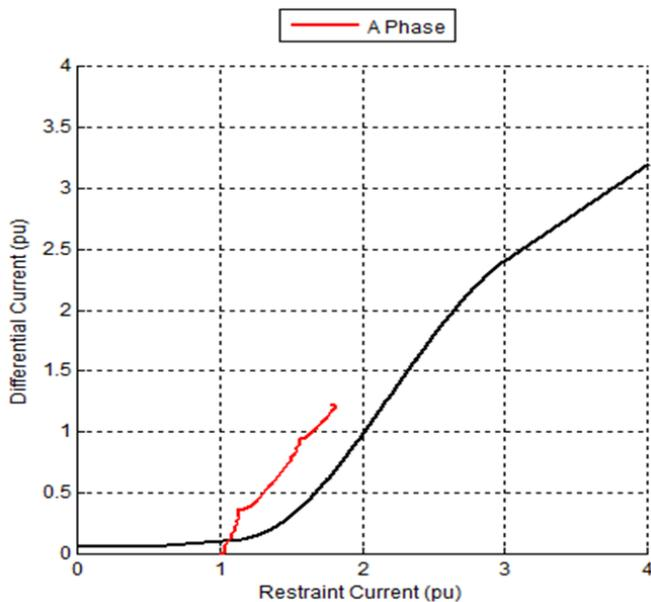
Fig. 2 Differential protection element during stator ground fault at 50% of the A-phase winding.
