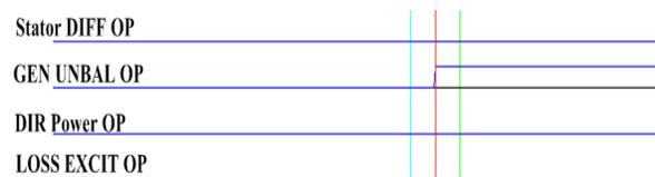
Fig. 5 Captured oscillography from an IED for inter-turn fault.
