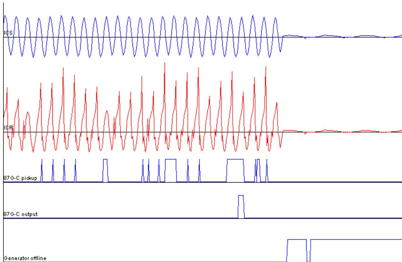
Fig. 13 Data captured for 87G digital generator protection relay.
