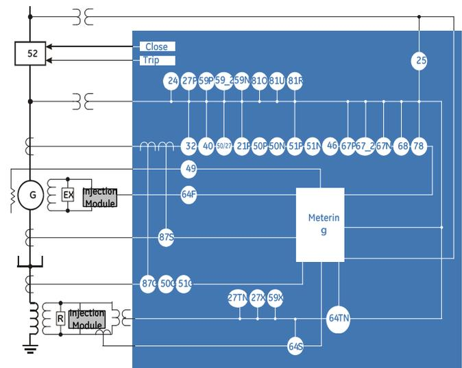
Fig. 1 A typical multifunctional generator protection system.
