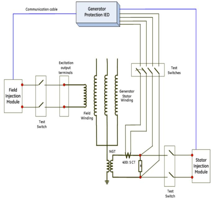
Fig. 7 Functional testing setup at Eastern Power, Canada.
