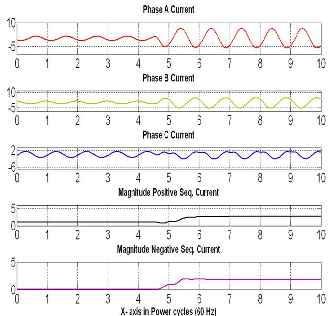
Fig. 4 Plot of generator terminal side currents and sequence components.
