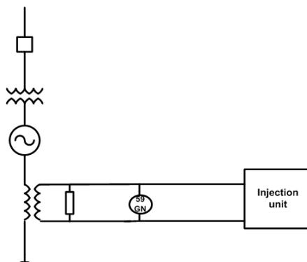
Fig 7. Stator Injection
