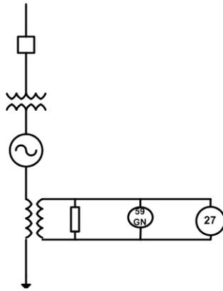
Fig. 5 Third Harmonic Undervoltage Relay
