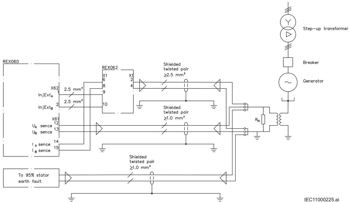
Fig 9. 100% Stator Connection
