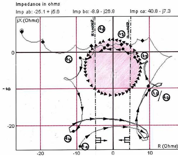
Figure 19. OST Function Characteristic Impedance Trajectory
