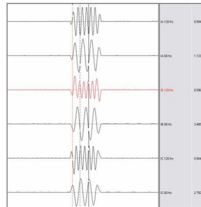
Figure 2. High Side CT Secondary Fundamental versus 2<sup>nd</sup> Harmonic Current
