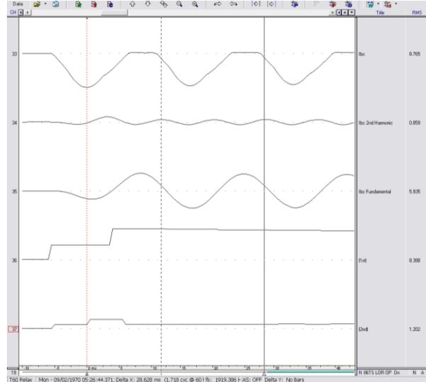
**Figure 5. Current Phasors Measured at the Relay with 2<sup>nd</sup> & 4<sup>th</sup> Harmonic Current**
