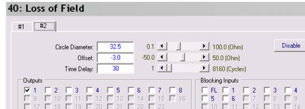
Figure 13. Loss of Field Zone 2 Impedance Settings
