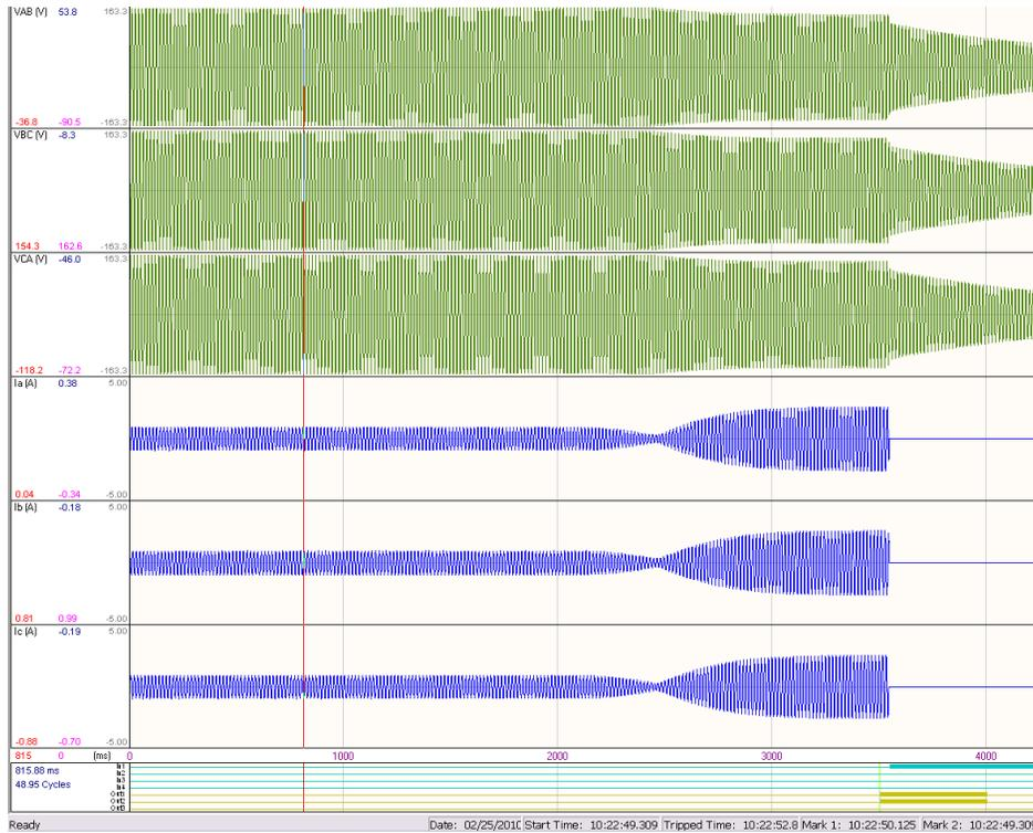
**Figure 9. Generator Loss of Field**
