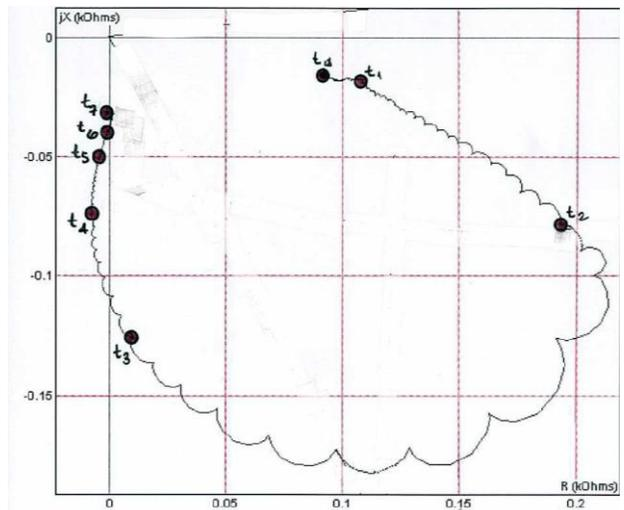
**Figure 10. Loss of Field Impedance Trajectory**
