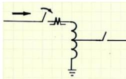
Figure 1. Auto Transformer Energization from High Side
