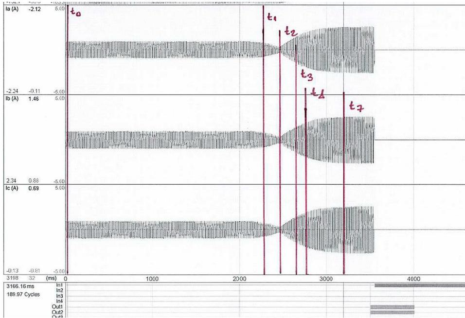
Figure 11. Loss of Field Current Channels
