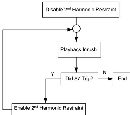
Figure 7. Transformer Inrush Test Procedure Flowchart
