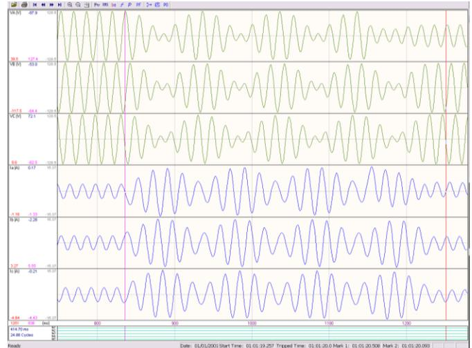
Figure 17. Out-of-Step (OST) followed by Single Line-to-Ground Fault
