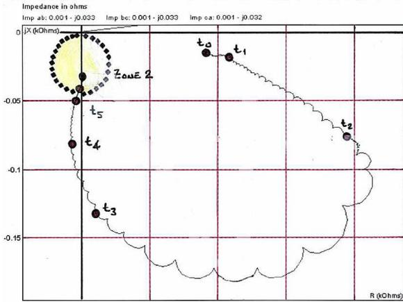
Figure 12A. Loss of Field Impedance Function Characteristic Impedance Trajectory
