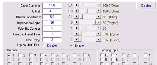
Figure 18B. Out-of-Step Impedance Settings
