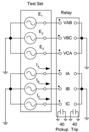
Figure 14. Test Connections
