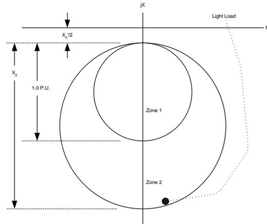
Figure 12B. Loss of Field Impedance Trajectory during Light Load
