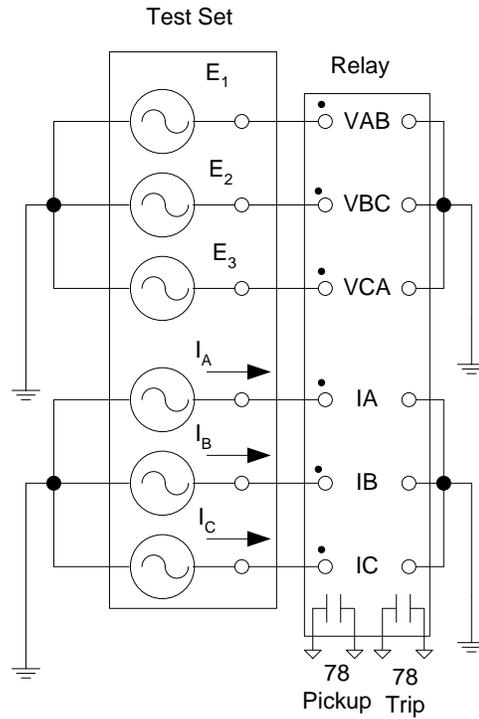
Figure 21. Test Connections
