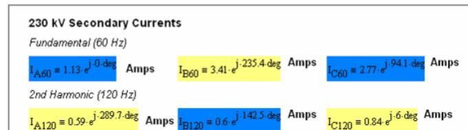
Figure 3. Current Phasors Measured at the Relay with 2<sup>nd</sup> Harmonic Current
