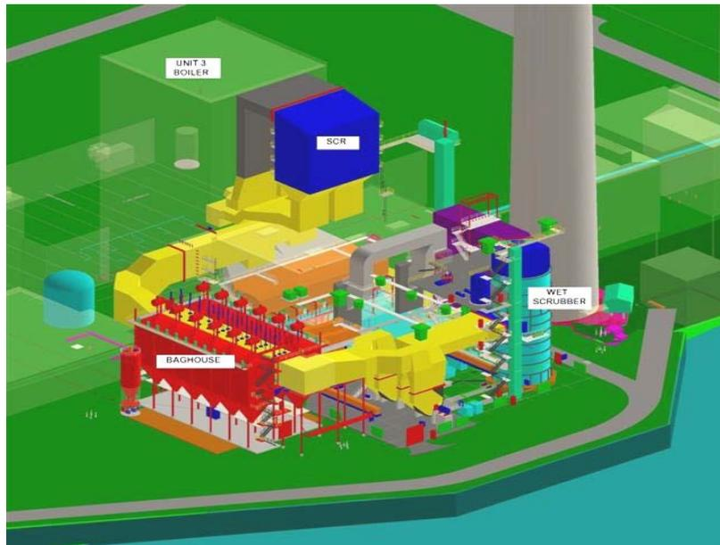
*Figure 1 – 3D Model of the Unit 3 Emissions Control Equipment.*
