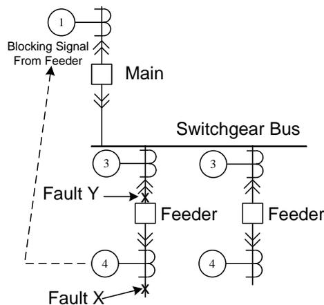
*Figure 7 – Bus Zone Tripping Scheme*
