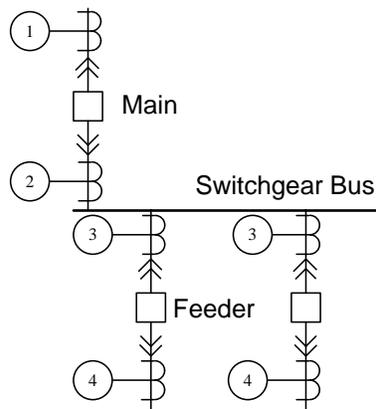
*Figure 6 – Typical Medium Voltage Switchgear Lineup*
