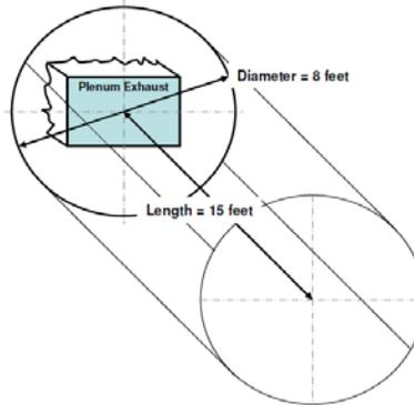
*Figure 5 – Plenum Exhaust Clearance Zone (Courtesy ABB)*
