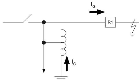
Fig. 15. Back-fed ground fault
