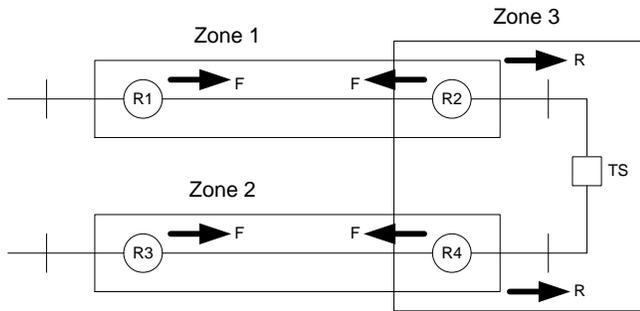
Fig. 13. Overlapping zones of protection
