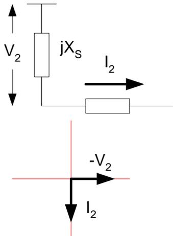
Fig. 18. Negative-sequence voltage polarized directional decision for forward fault (CCW rotation)
