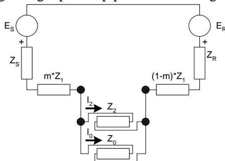
Fig. 17. Symmetrical component diagram for single-pole open
