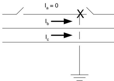
Fig. 16. A-phase tripped open
