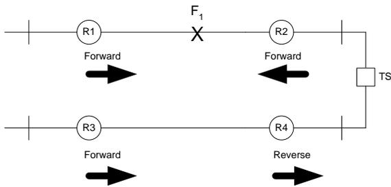
Fig. 8. Fault between reclosers R1 and R2
