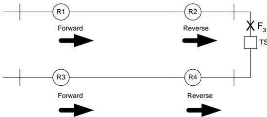
Fig 10. Fault between reclosers R2 and R4
