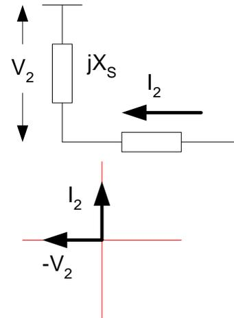
Fig. 19. Negative-sequence voltage polarized directional decision for reverse fault (CCW rotation)
