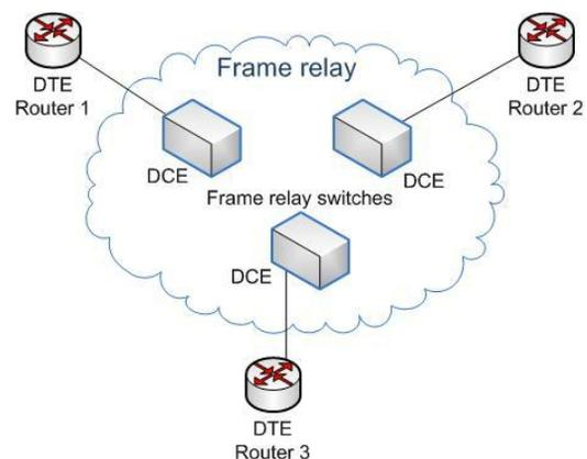
Fig. 1. Frame relay topology
