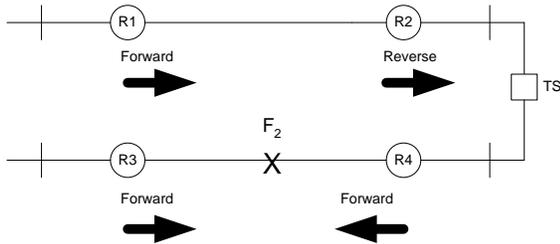
Fig. 9. Fault between reclosers R3 and R4
