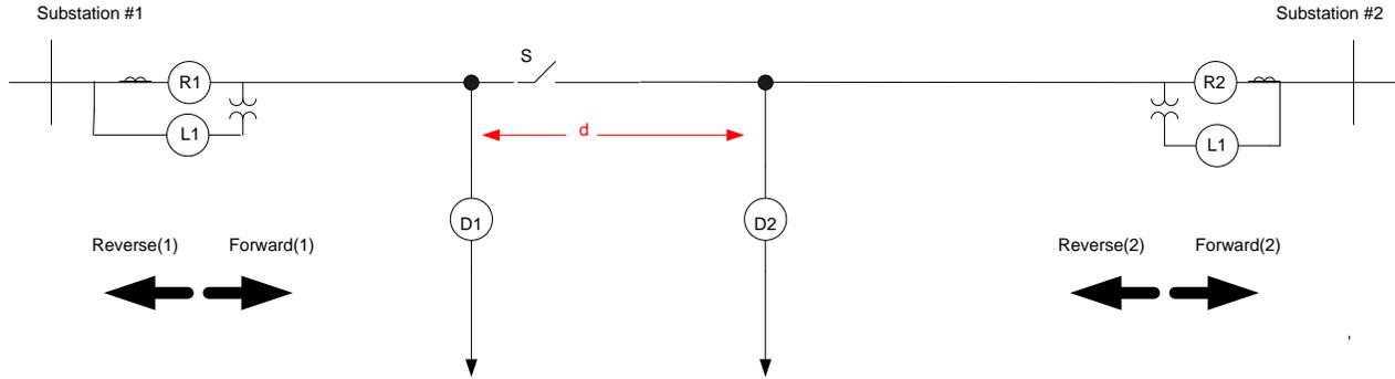
Fig 2. Single-line diagram for HSCAT scheme
