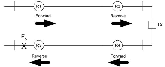
Fig. 12. Fault behind recloser R3
