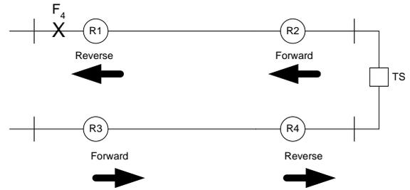
Fig. 11. Fault behind recloser R1
