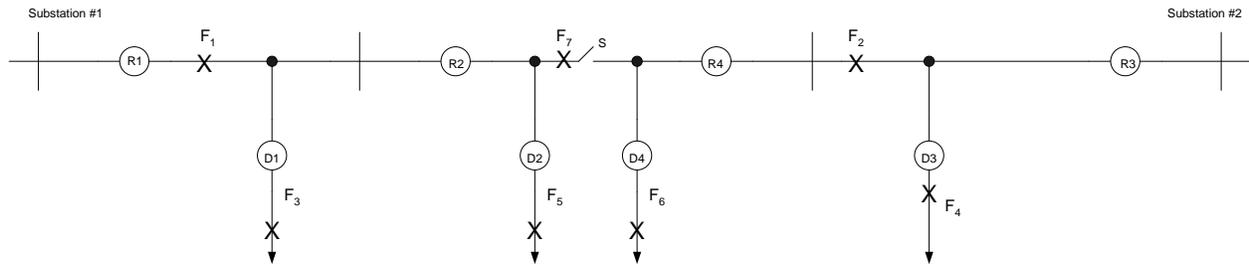
Fig. 14. Looped distribution system with sectionalizers
