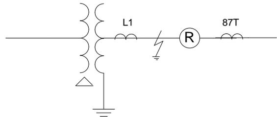
Fig 6. CT locations for bus faults
