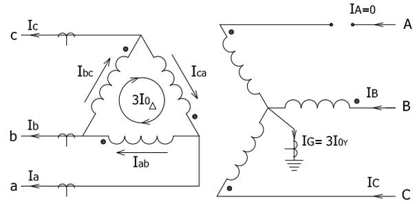
Fig. 21.  $Y_g$ - $\Delta$  Transformer with D11 Secondary Winding
