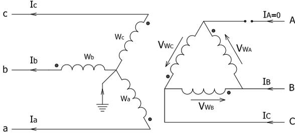
Fig. 14.  $\Delta$ - $Y_g$  Transformer with Phase A Open on the High Side
