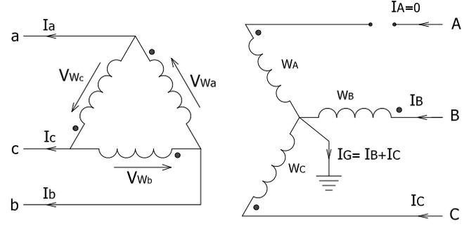
Fig. 9. Open Phase in a  $Y_g$ - $\Delta$  Transformer
