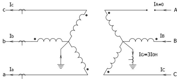
Fig. 26. Currents in a  $Y_g$ - $Y_g$  Transformer
