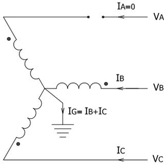
Fig. 6.  $Y_g$  Primary Winding with Phase A Open
