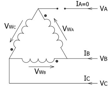
Fig. 7.  $\Delta$  Primary Winding with Phase A Open
