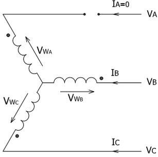
Fig. 8.  $Y$  Primary Winding with Phase A Open
