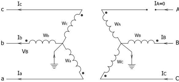
Fig. 16.  $Y_g$ - $Y_g$  Transformer With an Open Phase
