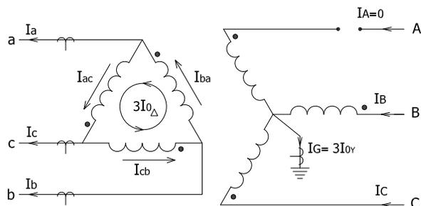
Fig. 20.  $Y_g$ - $\Delta$  Transformer with D1 Secondary Winding
